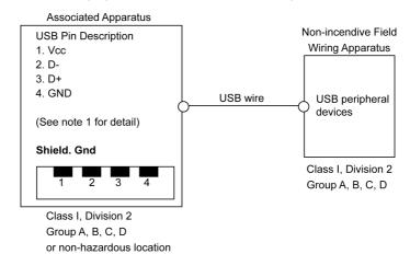
The following figure shows the USB cable wiring:
