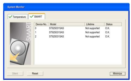
**NOTE:** In addition to the **Status** column, the **SMART** tab shows a column for the device lifetime. If the device has lifetime support, a **Lifetime** value in percent with a bar bargraph is displayed, otherwise "**Not supported**" is shown.
