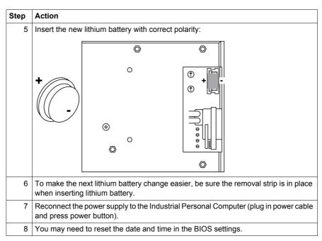
**NOTE:** Replacement of the lithium battery in the Industrial Personal Computer other than with the type specified in this documentation may present a risk of fire or explosion.
